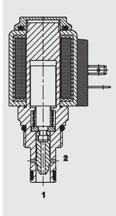
In the de-energized mode, the valve blocks flow in both directions. When energized the valve allows flow in both directions. **2/2 Solenoid Directional Valve UNE Spool Type, Direct-Acting SAE-08 Cartridge – 350 bar** WK08W-01
