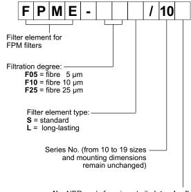
N = NBR seals for mineral oils (standard)V = FPM seals for special fluids (upon request)
